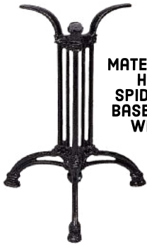
TT 106 MATERIAL: CAST IRON HEIGHT: 28.5" SPIDER LENGTH: 18" BASE SPREAD: 23.5" WEIGHT: 53LBS
