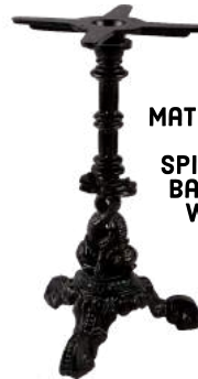
TT 104 MATERIAL: CAST IRON HEIGHT: 28" SPIDER LENGTH: 16" BASE SPREAD: 24" WEIGHT: 31LBS
