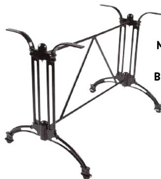
TT 106 EXT CA UMBRELLA BASE MATERIAL: CAST ALUMINUM HEIGHT: 28.5" SPIDER LENGTH: 27" BASE SPREAD: 34" WEIGHT: 25LBS
