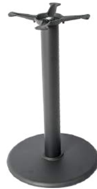
ECONOMY 18" ROUND MATERIAL: CAST IRON HEIGHT: 28" SPIDER LENGTH: 13" BASE SPREAD: 18" WEIGHT: 19LBS BAR HEIGHT AVAILABLE
