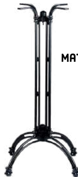
TT 106 EXT CA UMBRELLA BASE MATERIAL: CAST ALUMINUM HEIGHT: 28.5" SPIDER LENGTH: 27" BASE SPREAD: 34" WEIGHT: 25LBS
